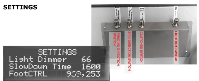
To get **access** to the setting menu, keep the *lightbox switch button* pressed when switching on the equipment.
